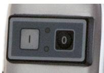
4 Press pushbutton **I** to switch on the machine (the light signal is illuminated)
